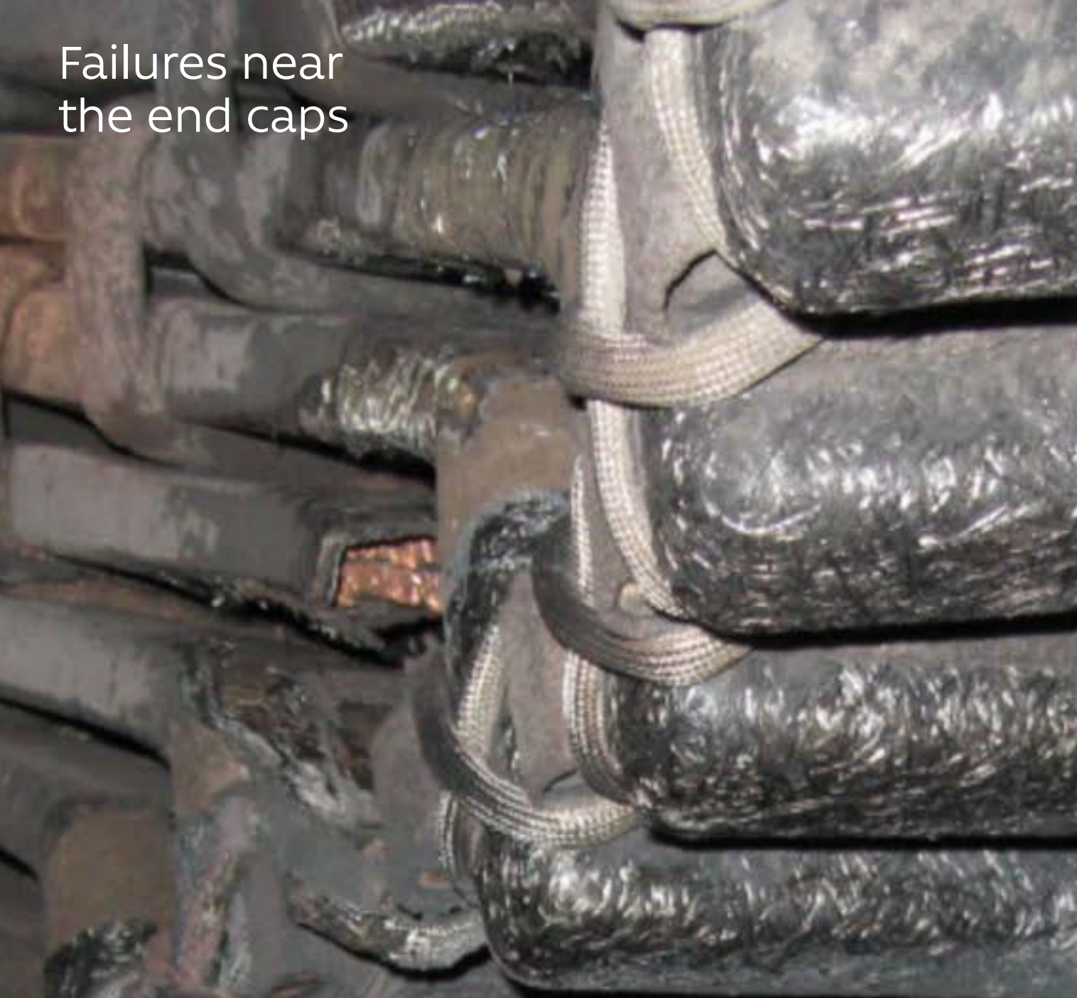
Build-up of contaminants at bottom of field slots and vent slots
