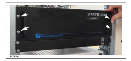
Slide the unit in the rack and use four screws on the front plate to hold it in place.
