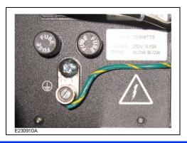
The protective conductor terminal must be connected to a grounding point in compliance with local regulations. Grounding is essential for safety purposes.
