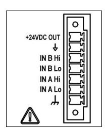
Each port is wired through a 7-position removable mini-connector which allows connection of signal input, shield, and +24VDC output for powering the measuring chain.
