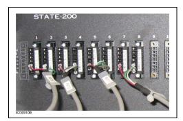
To remove a connector from an input port or the power input port, loosen the two screws securing the connector to the socket. If needed, use an extractor tool to pull a cabled connector off its socket. Do not pull on the wires.
