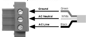
Note: In cabinets housing several instruments, it is common practice to connect only Line and Neutral. To prevent ground loops, only the protective conductor terminal gets connected to ground.
