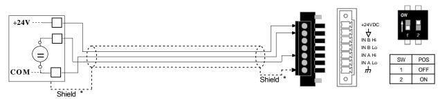
Note\*: To avoid ground loop problems, connect shield to earth ground on one end of the cable only.
