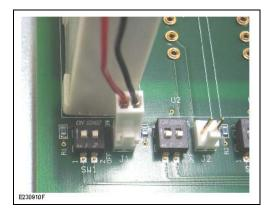
On the backplane, a small DIP switch and two pins are assigned to each module location.
