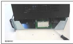
2. Open the casing of the STATE-200 unit by removing the 2 screws on each side holding down the cover.
