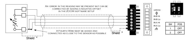
Note\*: To avoid ground loop problems, connect shield to earth ground on one end of the cable only.
