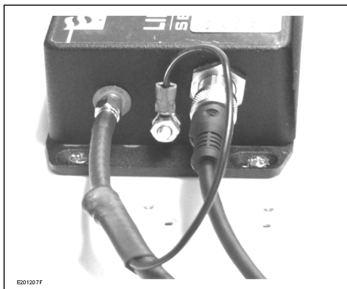
Figure 27 : Power and Signal output cable (right) connected to a LIN-300 Series module
