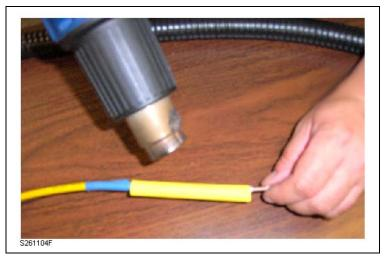
Figure 20 : Heating the heat-shrinkable tubing
