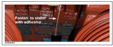
Figure 22 : Fastening integral cable to stator
