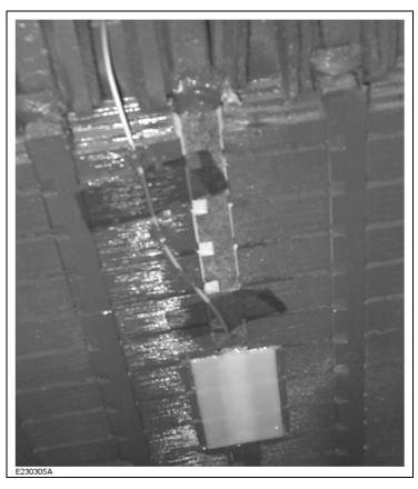
Figure 10 : Coaxial cable of a DCS-400 sensor temporarily taped to the stator
