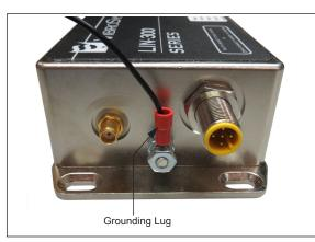
1. Make sure the grounding lug is firmly secured to the LIN-300's grounding terminal.
