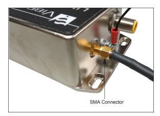
2. Make sure the extension cable's SMA connector is firmly secured to the LIN-300's SMA socket.
