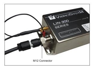
3. Make sure the M12 connector is firmly secured in place.
