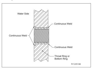
2. Using a continuous weld, weld the mounting adapter in place on both sides of the ring.
