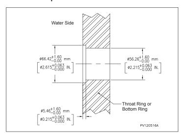
1. Drill the chamber into the ring.
