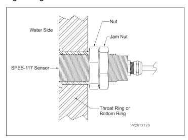
3. Complete by first tightening the nut, followed by the jam nut to secure the first in place.
