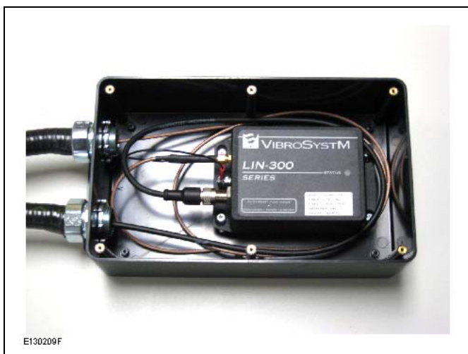
Figure 2 : Inside view of the ABS protection box
