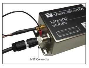
3. Make sure the M12 connector is firmly secured in place.
