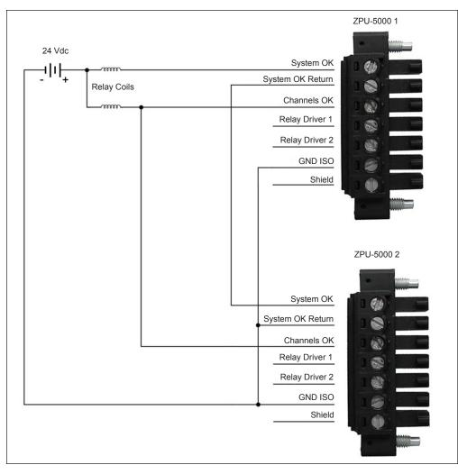
**Note:** Relay drivers 1 and 2 are available for optional configurations using the ZOOM software.
