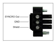
The SYNCHRO 1/Rev probe output connector is equipped with a 3position panel header with a threaded flange as well as a mating connector with a screw flange.
