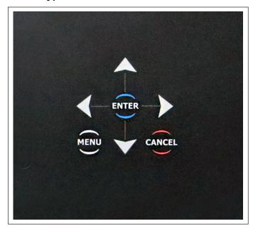
The **MENU** button is used for toggling in and out of **Menu** mode.
