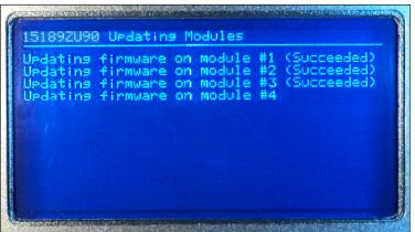
5. Once the operation is completed on a module, a message is displayed to confirm that the update was successful. If another module is installed, the updating program then proceeds with the next one.
