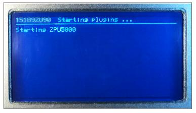
3. During Plug-in load up, the ZPU-5000 network address is displayed, represented by the acquisition unit's serial number.
