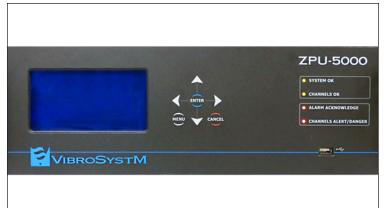
The VFD is blank and all LEDs light up for approximately 35 seconds in the following initial colors:
