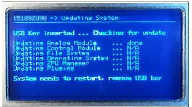
1. First, insert the USB key. The **SYSTEM OK** LED will blink Yellow during the data transfer.
