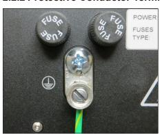
The protective conductor terminal must be connected to a grounding point in compliance with local regulations. Grounding is essential for safety purposes as well as to provide better efficiency against ESD and EMI disturbances.
