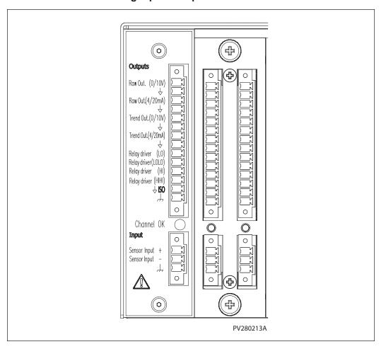
Analog input/output modules are two-channel electronic cards capable of converting input signals according to selected processes and generating corresponding analog signals. A ZPU-5000 unit can accept up to eight analog input/output modules. For each input channel, the data is processed according to the sensor's configuration in ZOOM. Processed raw and trend outputs are then available in both 4 to 20 mA and 0 to 10V formats for real-time monitoring.
