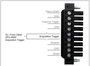
3. **Acquisition Trigger**: a bi-directional port used to allow a master ZPU-5000 unit equipped with an air gap sensor to share a 1/pole reference signal to slave ZPU-5000 units not equipped with an air gap sensor.
