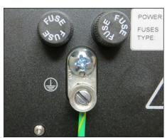
The protective conductor terminal must be connected to a grounding point in compliance with local regulations. Grounding is essential for safety purposes as well as to provide better efficiency against ESD and EMI disturbances.
