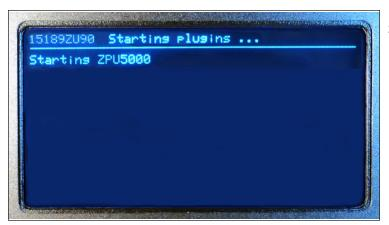
3. The ZPU-5000 network address is displayed, and all applicable service plug-ins are started. Square brackets around the ZPU-5000 network address indicate that the acquisition unit is not connected to the network yet.
