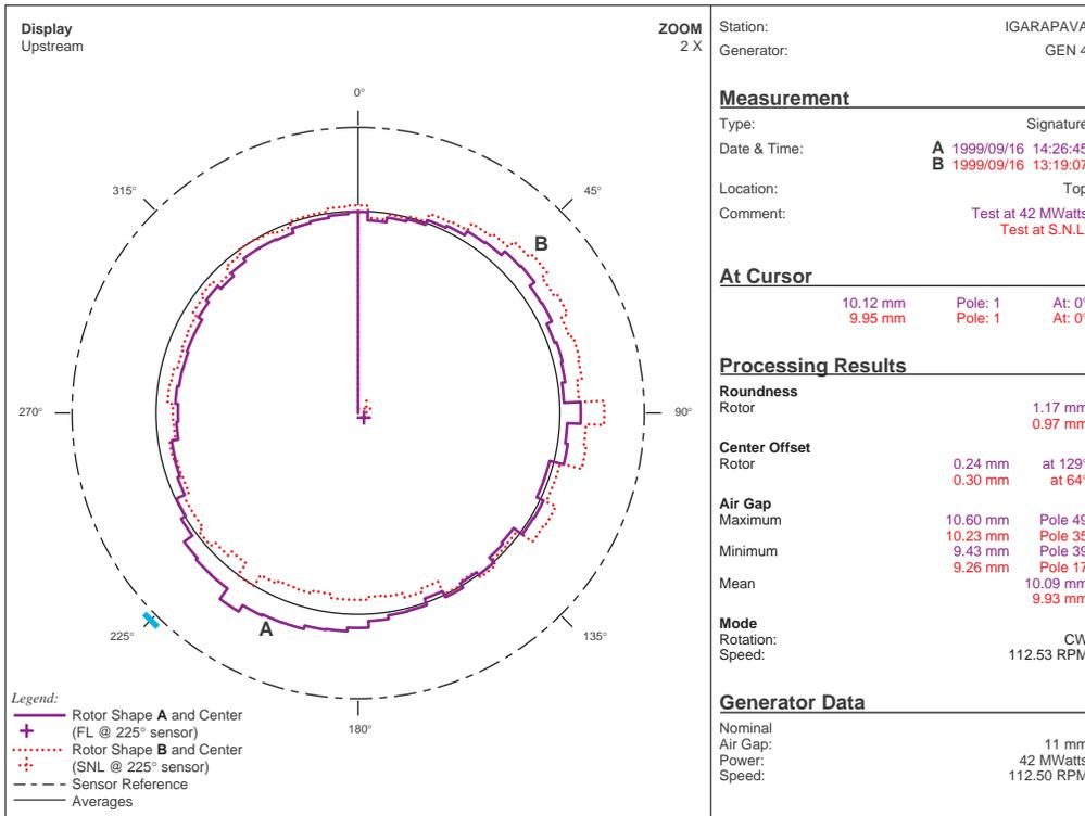
**Figure 5: Polar view of generator comparing rotor shapes at S.N.L. (B) and Full Load (A) using 225° sensor. Numerical values at right stress the various changes in roundness, offset, angle, best/worst locations.**
